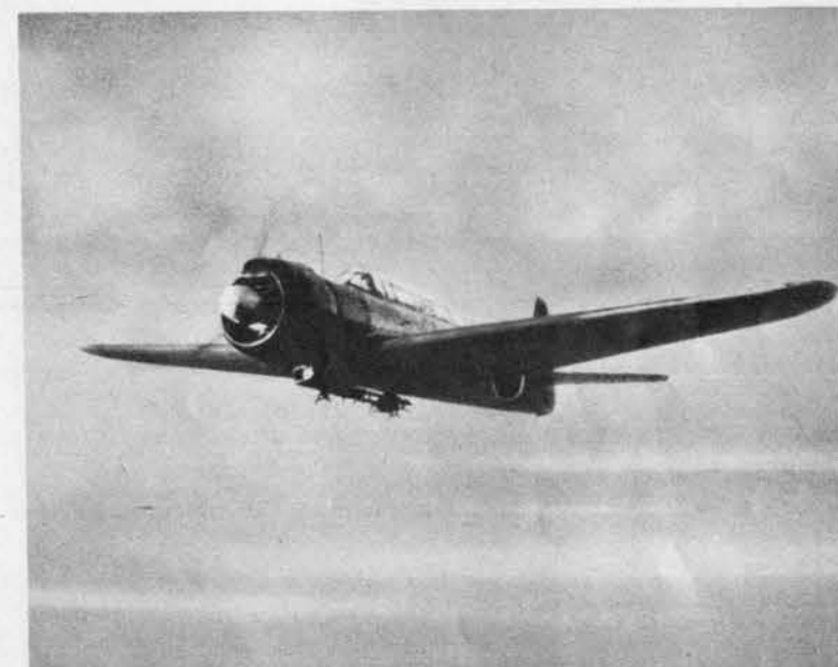
JILL Chief Japanese carrier-borne torpedo plane, Jill has largely replaced Kate. Wing has unbroken dihedral from the roots and flap guides on trailing edge. Tail assembly resembles Myrt's.
